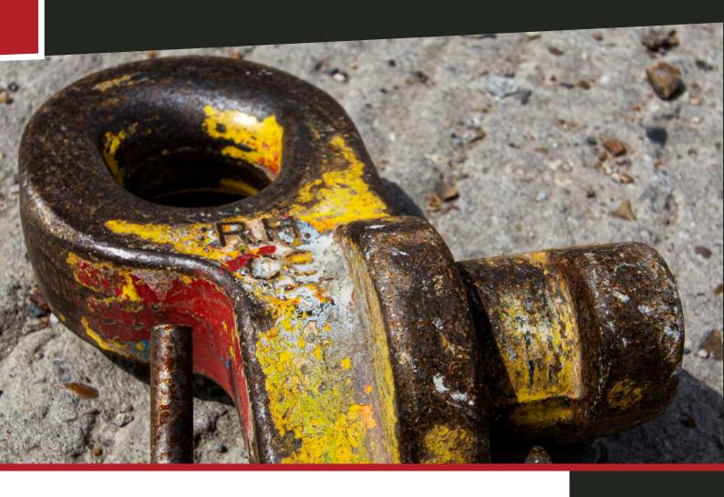
Shipping containers are designed to be lifted by ship to shore container cranes or port cranes using specialist lifting frames. But the reality is once a shipping container is inland there are many more occasions where they need to be lifted. The container lifting attachment, or shoe, provides a perfect, safe and easy solution.
