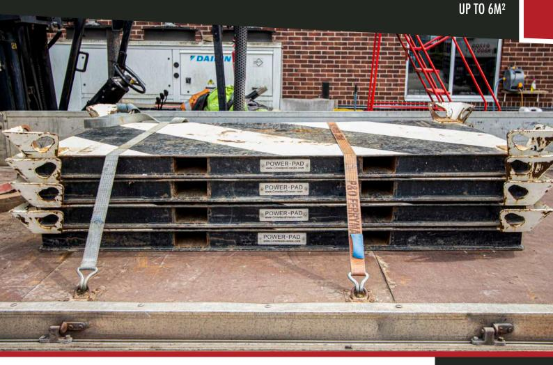
Poor ground conditions and incorrect outrigger mat selection is the main cause of accidents in the crane industry and that's why we stock a huge range of mats for all applications. With from  $0.25m^2$  up to  $6m^2$  in nylon, steel and timber, we can spread the load and reduce the ground bearing pressure to safe levels on almost any surface with even the biggest cranes.
