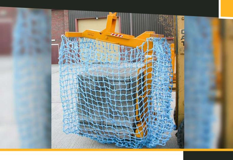
There are many ways to move or lift a pallet but this is the most safe and secure. When you have to lift a pallet onto a multi-story building or over a busy construction site using this system is the best way to ensure that there is no chance of falling debris and the pallet is delivered in exactly the same condition it left the ground.
