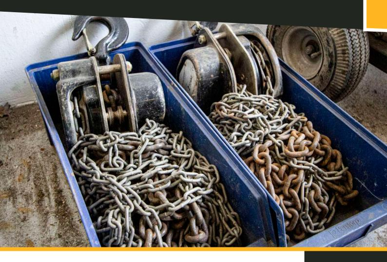
Chain blocks are a fantastic tool for lifting with precision. Loads with an uneven weight distribution or irregular lifting points can require fine adjustment to ensure the item is lifted safely and the chain block is the perfect piece of equipment for this.
