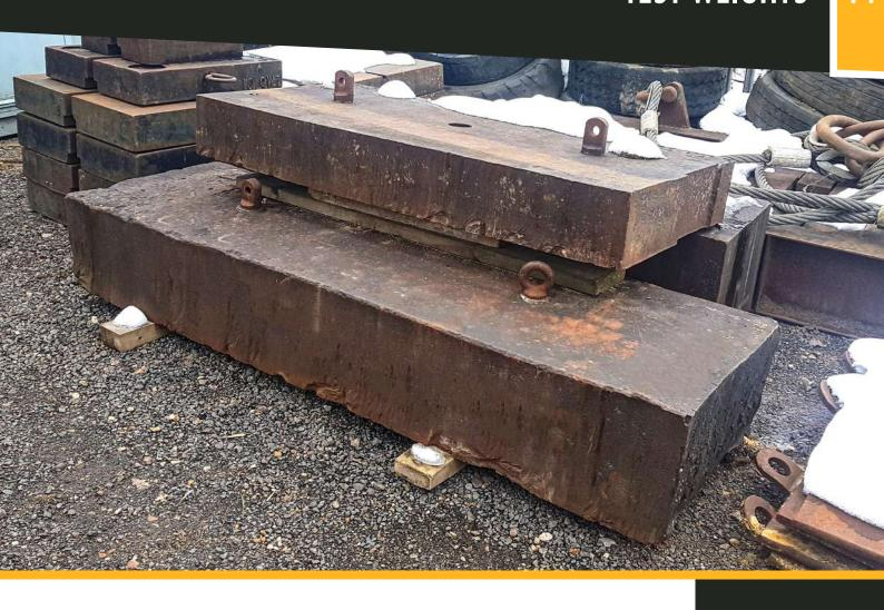
When manufacturing a new load bearing item it is necessary to apply 125% of the maximum stated capacity of the item. To do this you need test weights which can be anything from water, to sand to steel. Our steel test weights used in conjunction with our cranes offer a quick simple solution.
