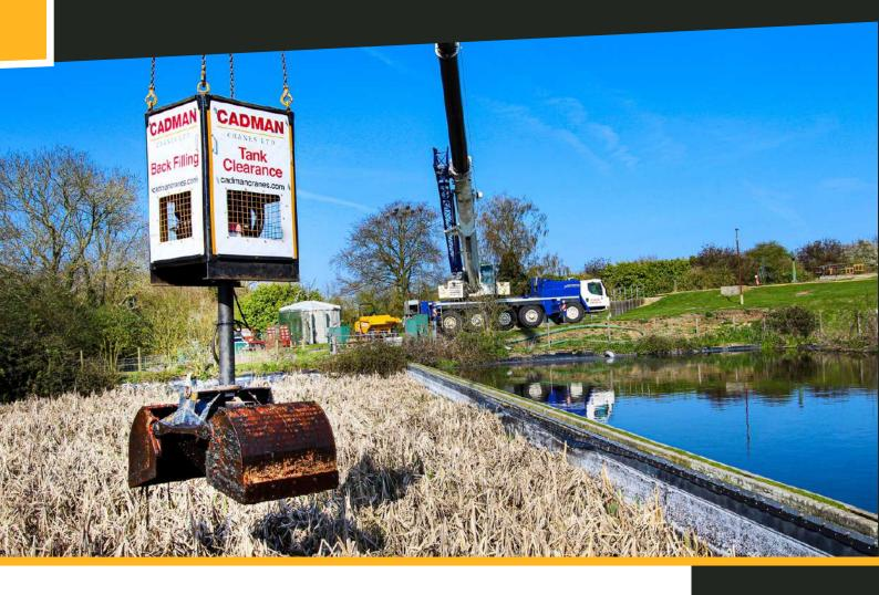
Our unique grab system can be used with any crane to achieve reaches of up to 70m. Designed specifically by Cadman Cranes for tank clearance in the waste water and anaerobic digestion industries this revolutionary piece of equipment provides a safer, quicker solution in a number of varied applications. Click here for more information.
