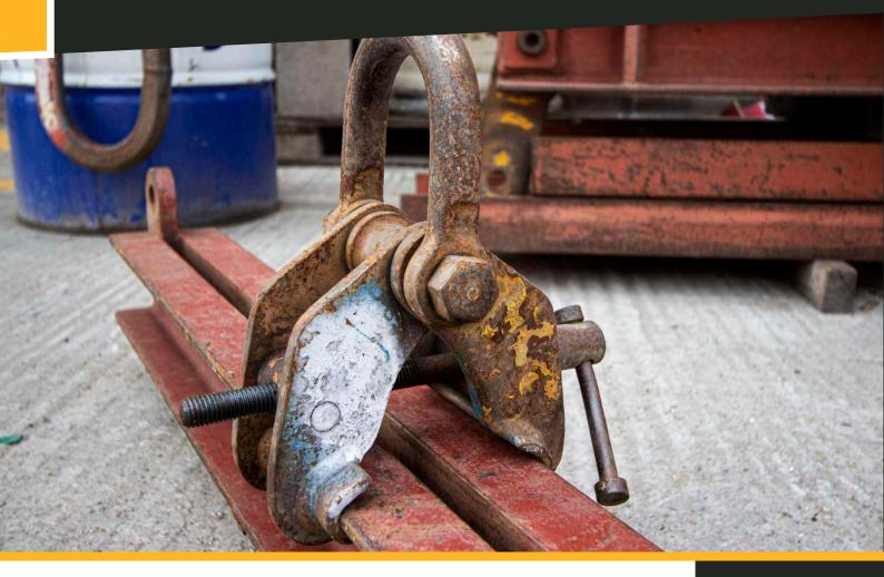
Working inside buildings can be tricky and one of the main reasons is the restricted headroom. A beam clamp is a great tool for reducing the height of the lift removing the need for chains or slings and allowing for direct attachment to the crane hook.
