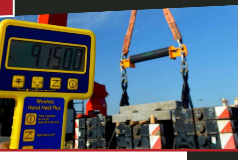
Sometimes our customers need to know the exact weight of the item being lifted. Modern cranes can do this through the onboard computer but for accuracy and piece of mind, nothing beats a calibrated load cell.
